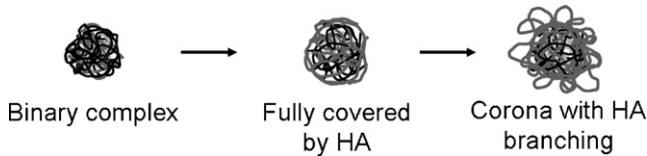
Fig. 5. Surface structure of the ternary complex coated by HA.
